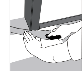
12 Door molding and skirting: lay a board (with the decorative side down) next to the door molding and as shown in the figure. Then slide the floorboard under molding.
